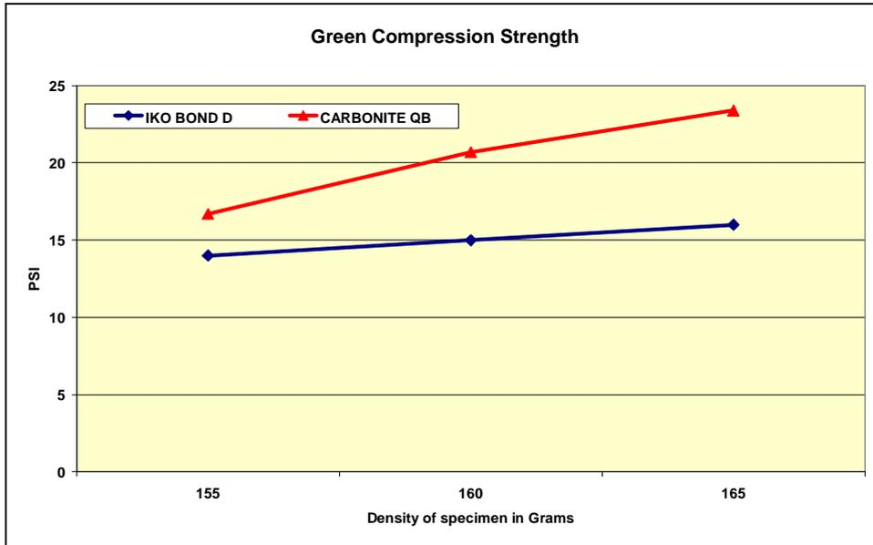
Figure 6, increased strength by using a “semi” organic modified bentonite (CARBONITE)
