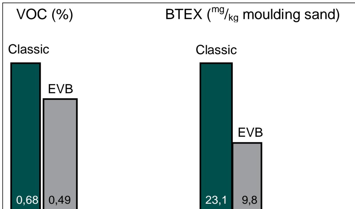
Figure 11, Emission reduction after introduction of ENVIBOND. Foundry is “core intensive”
