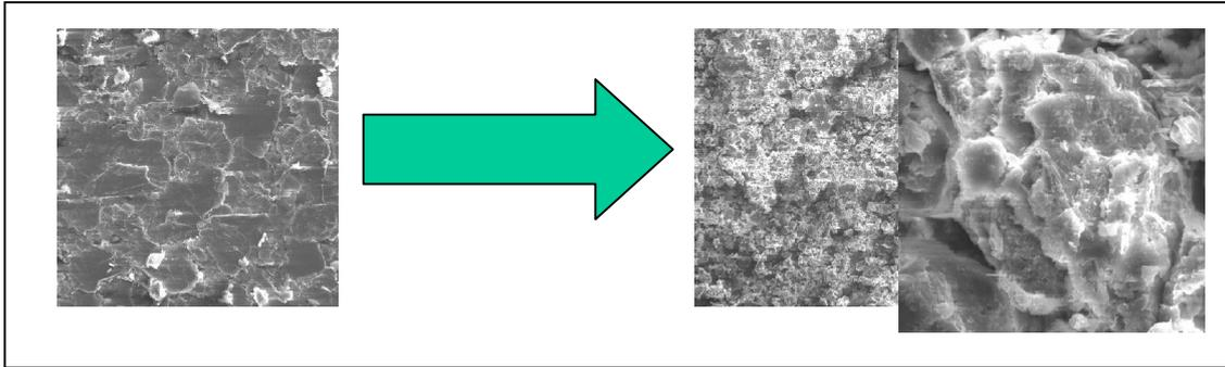
Figure 3, macro crystalline graphite when it is processed with bentonite creates a new bentonite (QUICKBOND) (pictures graphite left – QUICKBOND right)
