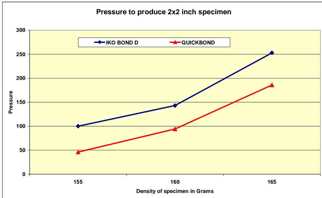
Figure 4, to achieve same density with process carbon modified bentonite (QUICKBOND) less pressure is required.
