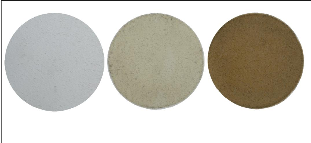
Figure 9, Foundry greensand, filters after test casting, left original, middle ENVIBOND, right classical foundry.
