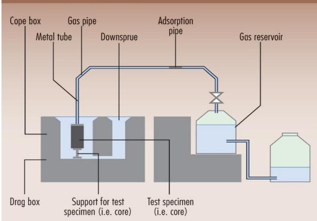
Figure 8, measurement of emissions, with adsorption pipe or filter to collect selected hazardous components, dust or condensates.
