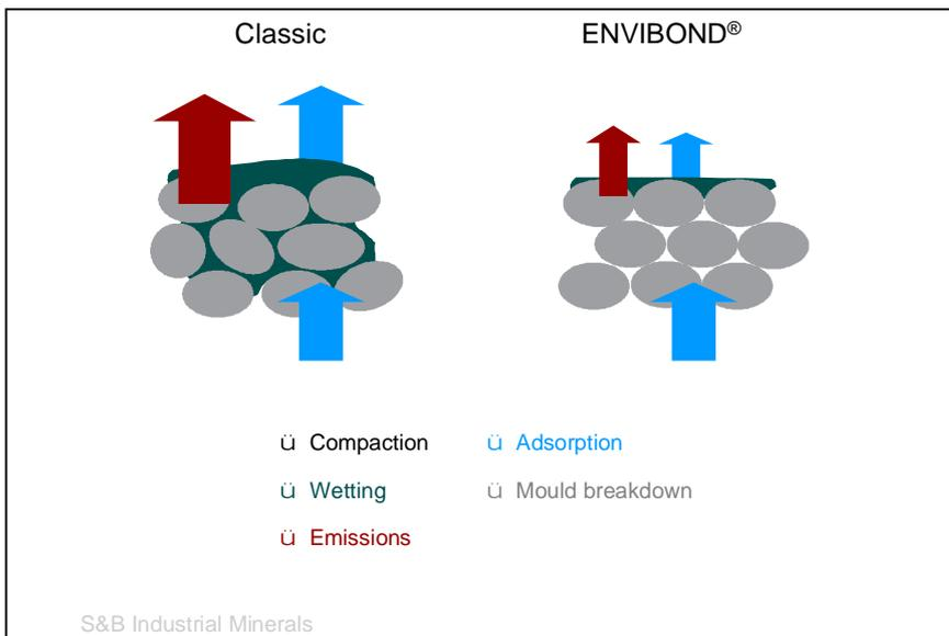
Figure 7, mechanism of ENVIBOND, higher compacted (less pores), less wetting by liquid metal, less carbonaceous additives (emissions), more adsorption (core binder gasses), good mold collapsing (shake out)
